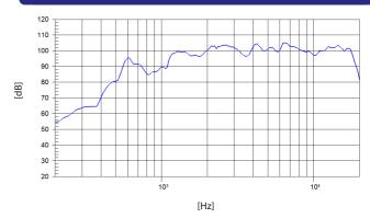
Note: On axis frequency response measured in anechoic chamber, 1W / 1m
